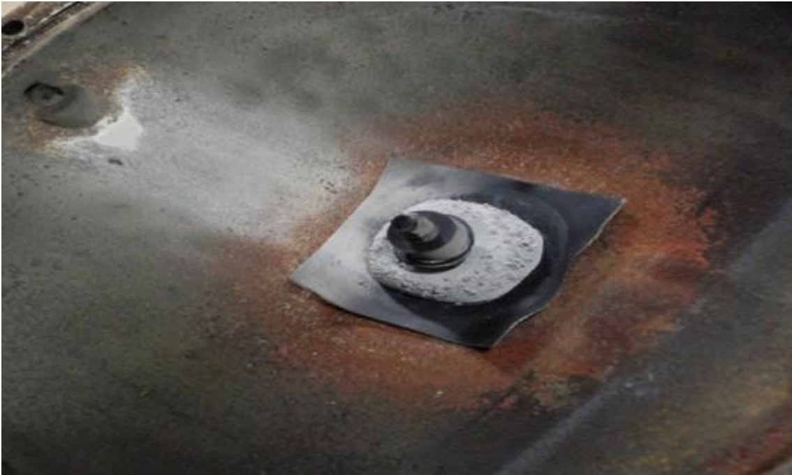
Chiller lid from phase one test facility after two cooling seasons on ProMoss™.
